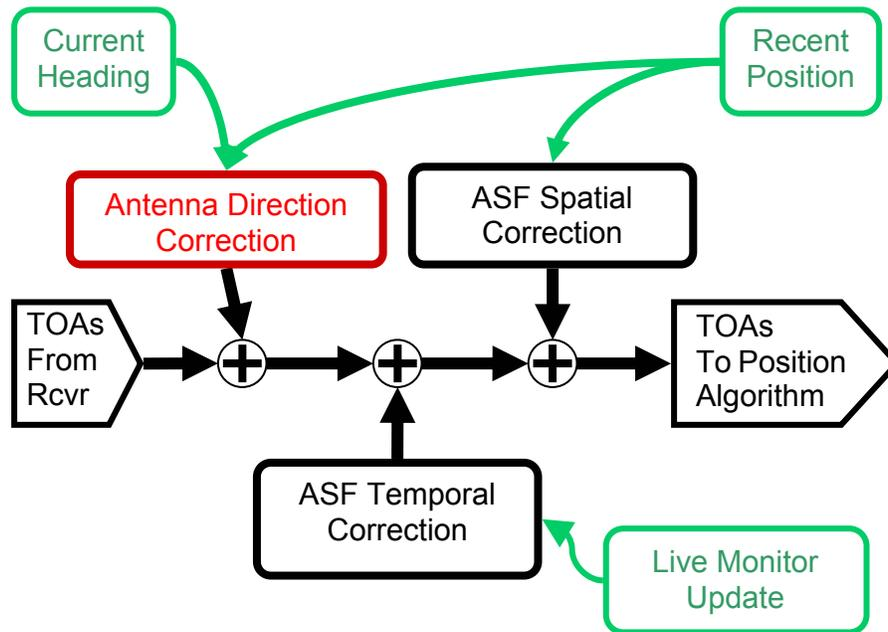
*Figure 1 – Block diagram of the enhanced Loran system.*
