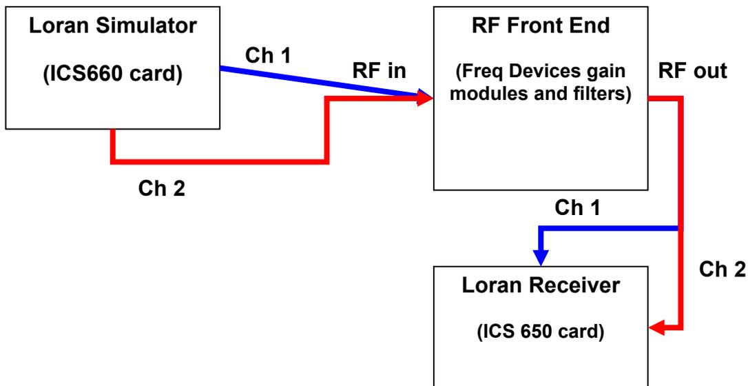
*Figure 15 – Simulating the effects of receiver time delays*
