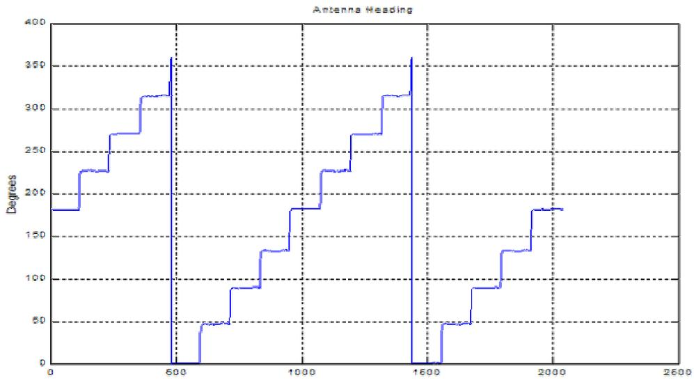
**Figure 20 – Antenna rotation headings, 45 degree steps.**
